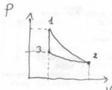
$$\eta = \frac{Q_{ess} - Q_{ad}}{Q_{ess}}, Q_{ess} = mc_v(T_1 - T_3), Q_{ad} = -L_{isot} = mRT_2 \ln \frac{V_2}{V_3} \Rightarrow$$
